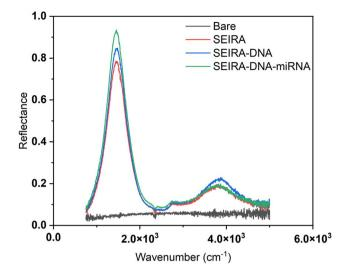
Fig. 5 SEIRA enhancement. Reflectance measurements of a bare area without SEIRA, shown as black, an area with SEIRA structures when it was clean (red), after DNA binding (blue), and after miRNA binding (areen).
