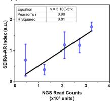
Fig. 6 SEIRA-AR measurements of hsa-miR-let-7a-5p correlation with (a) RT-qPCR and (b) NGS results. The mean and standard deviation values are in blue, and the fitted line is in black. The curve fitting parameters, including the fitting equation, Pearson's *r* value, and *R* Squared values, are shown in the top left corner.
