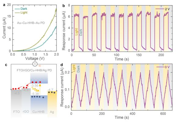
Fig. 2 (a) Current-voltage curves of Au-Cu-HHB-Au PD in dark and light. (b) Current-time response of the Au-Cu-HHB-Au PD under alternating dark and light conditions at 2 V applied bias (V = 2 V). (c and d) Energy band diagram of FTO/rGO/Cu-HHB/Ag PD and respective current-time curve of the PD under alternating dark and light illuminated conditions in the absence of external bias voltage (V = 0 V).
