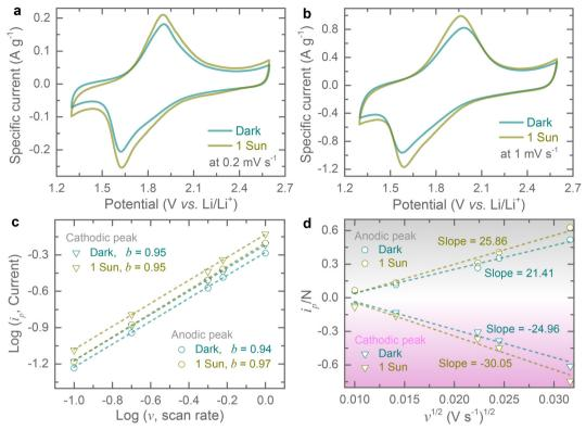
Fig. 3 Electrochemical performance of Cu-HHB electrodes both in the dark and 1 sun illuminated conditions. (a and b) CV profiles at 0.2 mV s<sup>-1</sup> and 1 mV s<sup>-1</sup> in the dark and 1 sun illumination. (c) Plots of log ( $i_p$ ) vs. log (v): estimation of b-values for cathodic and anodic peaks in the dark and 1 sun illumination. (d) Estimation of Li-ion diffusion constant improvements under illumination from  $I_p/N$  vs.  $v^{1/2}$  curves.
