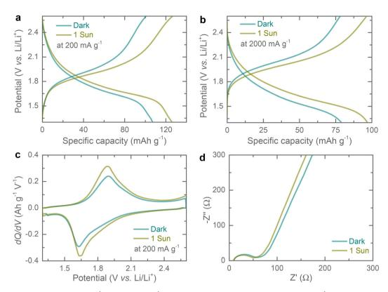
Fig. 4 (a and b) GDC profiles at 200 mA  $g^{-1}$  and 2000 mA  $g^{-1}$  and (c) the respective dQ/dV curves at 200 mA  $g^{-1}$  in the dark and 1 sun illuminated conditions. (d) Nyquist plots of the Ph-LIB in the dark and 1 sun conditions. EIS results were recorded in the frequency range of 10 mHz – 100 kHz at 10 mV amplitude after the 2nd galvanostatic discharge cycle to 2 V.
