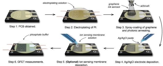
Fig. 2 The manufacturing process to make four-terminal graphene PCB transistors for chemical sensing.
