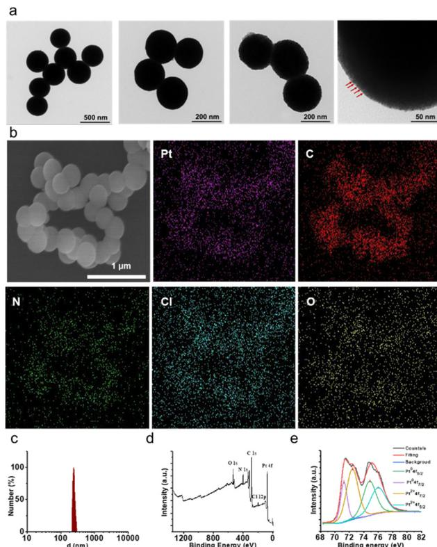
Fig. 2 Characterization of PNAs. (a) Representative TEM images of prepared PNAs. (b) Representative SEM and elemental mapping images of prepared PNAs. (c) DLS pattern of PNAs. (d) and (e) XPS spectra of PNAs (Pt<sup>2+</sup>: 4f7/2 brown; Pt<sup>2+</sup>: 4f5/2 blue; Pt (0): 4f7/2 purple; Pt (0): 4f5/2 green).
