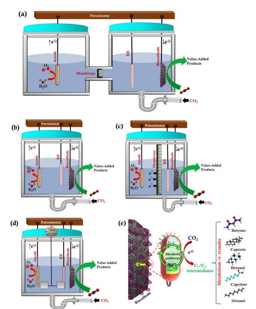
Fig. 2 Reactor configurations for MES-based CO<sub>2</sub> conversion: (a) H-type, (b) single chamber, (c) dual chamber, (d) continuous stirred tank, and (e) schematic of electron transfer mechanism
