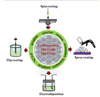
Fig. 3 Schematic of the fabrication of carbonaceous electrode materials.
