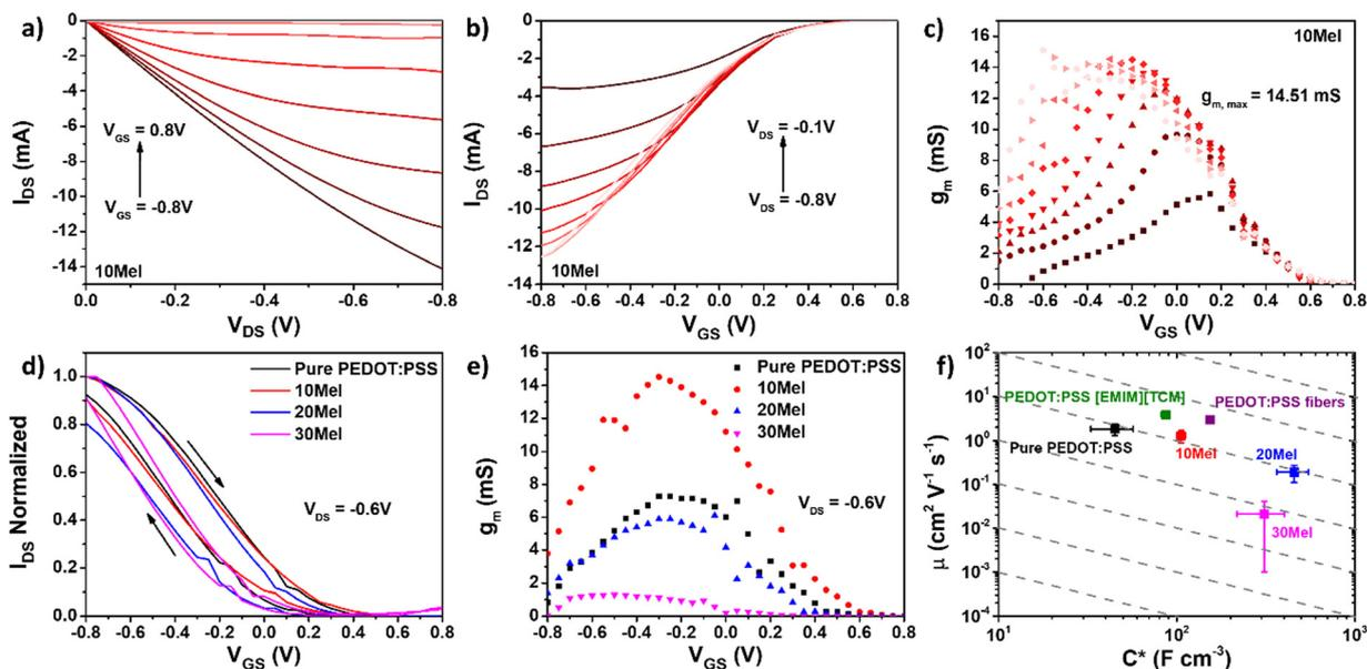
Fig. 6 (a) Output, (b) transfer, and (c) transconductance ( $g_m$ ) curves of 10Mel OECT. (d) Normalized transfer curves and (e)  $g_m$  curves for devices having various ratios of Mel/PEDOT:PSS. (f)  $\mu$  vs.  $C^*$  of OECTs based on different Mel/PEDOT:PSS ratios and reference literature values for other relevant PEDOT:PSS-based OMIECs.
