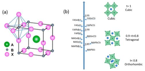
Fig. 1 (a) A sketch of the typical ABX<sub>3</sub> perovskite structure. (b) Tolerance factor along with perovskite distortion as a function of composition, from orthorhombic to cubic. Reproduced from ref. 46 with permission from Elsevier, copyright 2014 under a Creative Commons Attribution 4.0 International License (CC BY 4.0).
