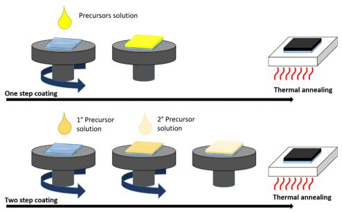
Fig. 4 Schematic description of one-step and two-step coating deposition
