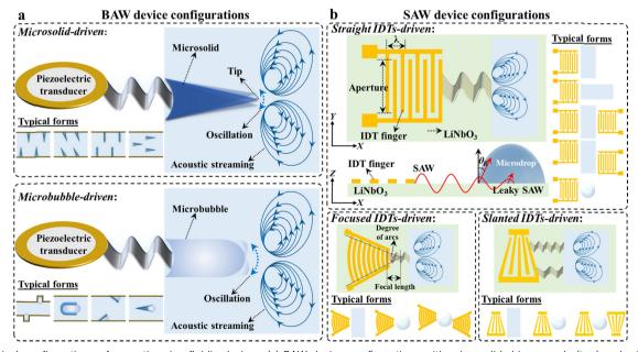
Fig. 2 Typical configurations of acoustic microfluidic devices. (a) BAW device configurations with microsolid-driven mode (top) and microbubbledriven mode (bottom); and (b) SAW device configurations with straight IDTs-driven mode (top), focused IDTs-driven mode (bottom-left), and slanted IDTs-driven mode (bottom-right).
