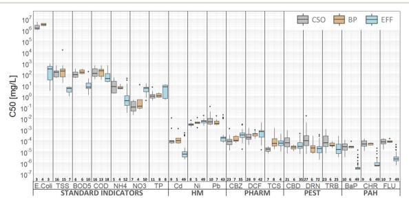
Fig. 2 Boxplots of median concentrations detected in each monitored IUWS per discharge type. The number of available data (i.e., number of IUWS) for each combination of discharge type and (micro-)pollutant is reported at the bottom of the graph. E. coli values refer to CFU/100 mL.
