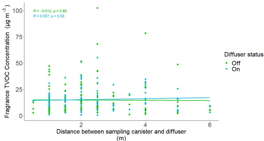
Fig. 4 The relationship between the sum of fragrance VOCs and the distance between the sampling canister and the fragrance diffuser. Regression statistics were calculated using a linear model.
