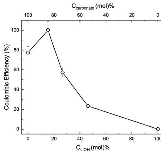
Fig. 13 Effect of initial LiOH content ( $C_{\text{LiOH}}$ , mol%) and initial carbonate content ( $C_{\text{carbonate}}$ , mol%) of the  $\text{Li}_2\text{CO}_3/\text{K}_2\text{CO}_3/\text{LiOH}$  electrolyte on the Coulombic efficiency of  $\text{CO}_2$  electro-splitting process at  $500^\circ\text{C}$ . The electrolyte  $\text{Li}_2\text{CO}_3/\text{K}_2\text{CO}_3$  mol ratio was set at eutectic 1.63 throughout.<sup>51</sup>
