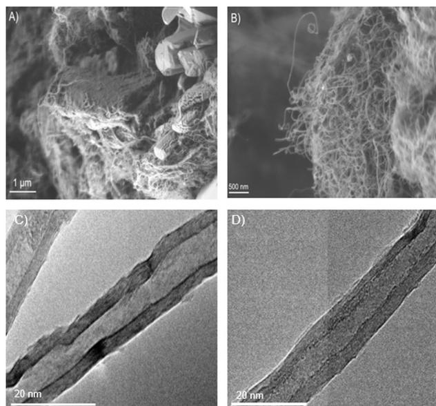
**Fig. 14** Top row: Representative SEM images of product obtained by electrolyzing  $(\text{Li}_{0.62}\text{K}_{0.38})_2\text{CO}_3$  + 13 mol% LiOH with 8 wt% LDPE at 14.2k $\times$  magnification (A) and 20.2k $\times$  (B). Bottom row: Representative TEM images of product obtained by electrolyzing  $(\text{Li}_{0.62}\text{K}_{0.38})_2\text{CO}_3$  + 13 mol% LiOH with 8 wt% LDPE (C) and the same with 8 wt% seaweed (D), confirming multiwalled carbon nanotubes.
