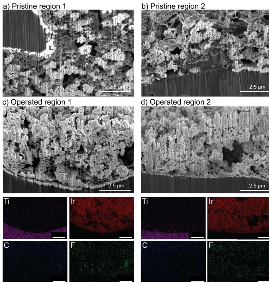
Fig. 9 Cross-sectional analysis of IrO<sub>x</sub>/mixed binder anode PTE. SEM images of different regions of the pristine catalyst layer (a) and (b) and SEM with EDX maps of two operated regions (c) and (d). Only PTFE binder is observed in the catalyst layer after operation.
