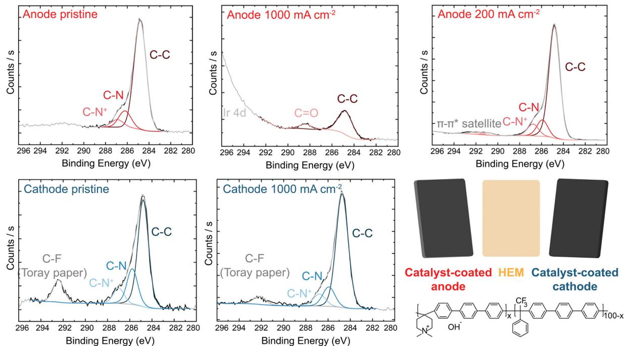
Fig. 4 XPS analysis of IrO<sub>x</sub>/20% TP-85 anode and Pt-black/10% TP-85 cathode. C 1s spectra of (a) anode and (b) cathode PTE. Inset shows the chemical structure of the TP-85 ionomer. Ionomer degradation is only observed on the anode PTE operating at high current.
