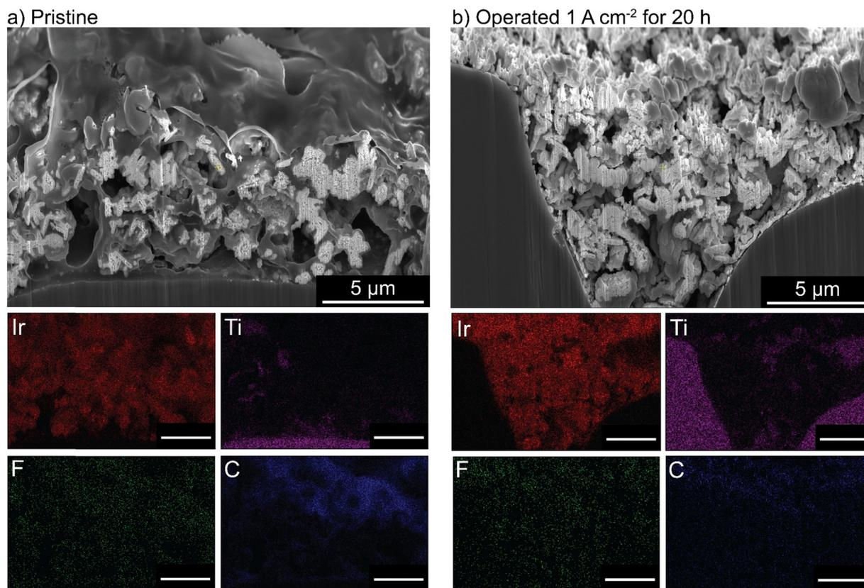
Fig. 5 Cross-sectional imaging and EDX of an IrO<sub>x</sub>/20% TP-85 anode PTE. (a) Before and (b) after 20 h operation at 1 A cm<sup>-2</sup>. All scale bars are 5 μm. No ionomer is observed in the catalyst layer after operation.
