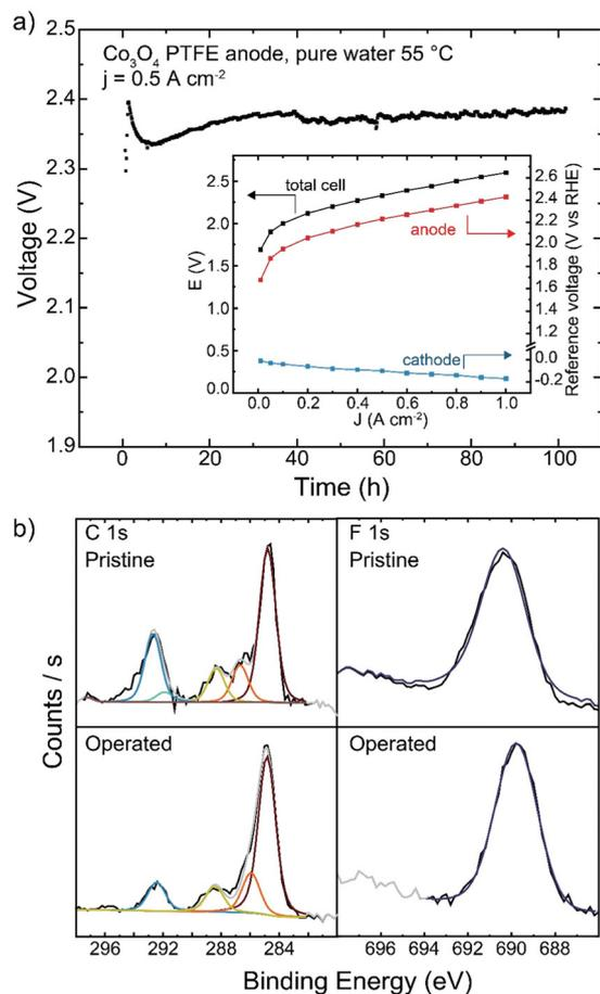
Fig. 10 Long-term operation of a PTFE-containing anode. (a) HEM electrolyzer operation with a  $\text{Co}_3\text{O}_4/20\%$  PTFE-coated stainless-steel anode PTE, TP-85 membrane, and Pt-black/10% TP-85 cathode for 100 h at 55 °C. Inset shows cathode and anode contributions to total cell voltage. (b) XPS of the anode catalyst layer before and after 100 h operation.
