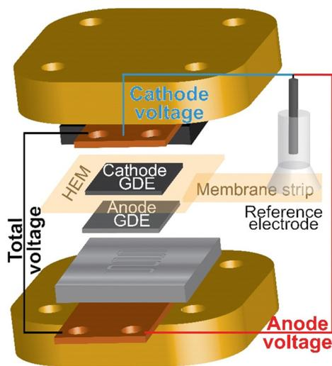
**Fig. 2** Schematic of the reference electrode integrated in the electrolyzer MEA and hardware. A reference electrode is placed on a strip of membrane attached to the HEM in the MEA. The voltage is measured from the cathode end plate or anode end plate *versus* the reference. Precision gasketing and a high-conductivity HEM reference strip are used to minimize misalignment reference-potential errors.<sup>48,49</sup>
