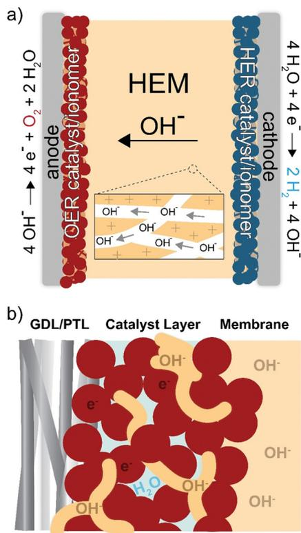
Fig. 1 Ion transport and reactivity in HEM electrolyzers. Schematics of (a) electrolyzer cell and (b) anode-catalyst layer. The  $\text{OH}^-$  anions conduct through the ionomer, and electrons conduct through the catalyst. Oxygen evolution occurs at the ionomer/catalyst interface.
