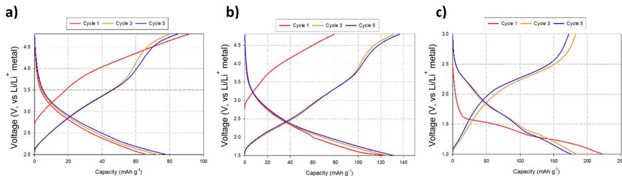
Fig. 8 Voltage profiles for BM- $\text{Li}_2\text{MoO}_4$  using varying voltage ranges: (a) 4.8–2.0 V, (b) 4.8–1.5 and (c) 3.0–1.0 V. Note: cell c was discharged first before charging to higher voltages.
