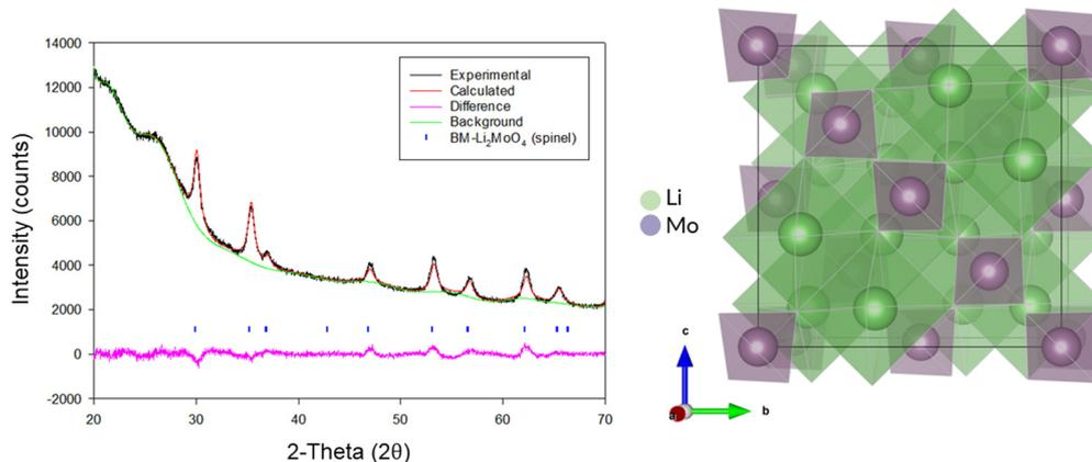
Fig. 2 Observed, calculated and difference profiles for Rietveld refinement of BM- $\text{Li}_2\text{MoO}_4$  (16 h) (left) and an image of the spinel structure adopted by this phase (right). (Cu  $K\alpha$ ).
