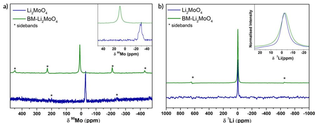
Fig. 3 (a)  $^{95}\text{Mo}$  NMR for  $\text{Li}_2\text{MoO}_4$  and BM- $\text{Li}_2\text{MoO}_4$  at 700 MHz (16.4 Tesla), 10 kHz MAS, single pulse spectra. (b)  $^7\text{Li}$  NMR at 200 MHz (4.7 Tesla), 50 kHz MAS, with 1  $\mu\text{s}$  pulse for  $\text{Li}_2\text{MoO}_4$  and BM- $\text{Li}_2\text{MoO}_4$ . In both figures, inset focuses on the central transition peak.
