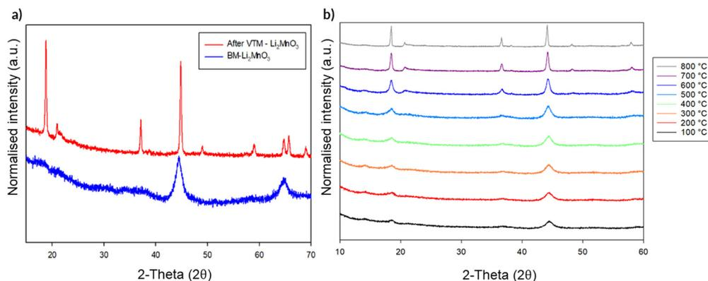
Fig. 11 (a) PXRD of BM-Li<sub>2</sub>MnO<sub>3</sub> sample before (DRS phase) and after VT-PXRD (layered phase) (b) VT-PXRD experiment in the region of 100–800 °C showing the change in the relative intensity of peaks with increasing temperature indicating a transformation from DRS to layered on heating. (Cu K $\alpha$ ).
