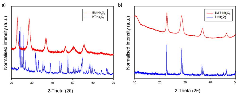
Fig. 14 (a) High temperature (HT) phase – H-Nb<sub>2</sub>O<sub>5</sub> before and after milling (BM) showing a phase conversion to T-Nb<sub>2</sub>O<sub>5</sub>. (b) Low temperature phase (T-Nb<sub>2</sub>O<sub>5</sub>) before and after milling showing no change in structure, just broadening of the peaks due to the smaller particle size after milling. (Cu K $\alpha$ ).
