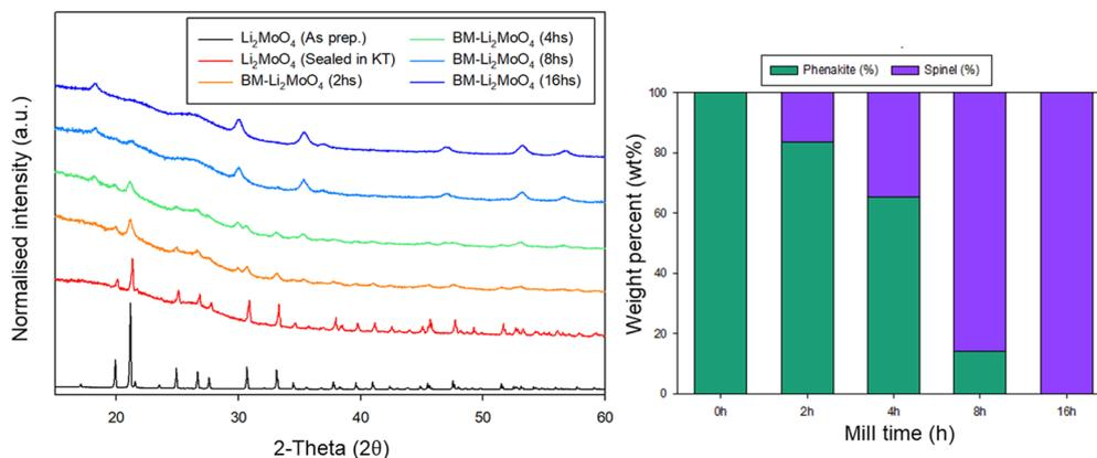
Fig. 1 PXRD of samples prior to and after milling illustrating a transformation from phenakite to spinel structure (left), with the calculated phase fractions from Rietveld refinement (right). (Cu  $K\alpha$ ). Note: the high background in samples after milling can be attributed to the Kapton tape (KT) used to measure the material to prevent air exposure.
