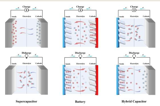
Fig. 2 Mechanisms of supercacitors, batteries and hybrid capacitors.
