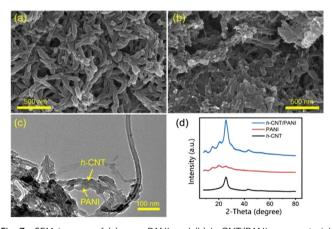
Fig. 7 SEM images of (a) pure PANI and (b) h-CNT/PANI nanomaterial. (c) TEM image of h-CNT/PANI nanomaterial. (d) XRD patterns of h-CNTs, pure PANI and h-CNT/PANI nanomaterial. 47 Reused with permission from Elsevier.
