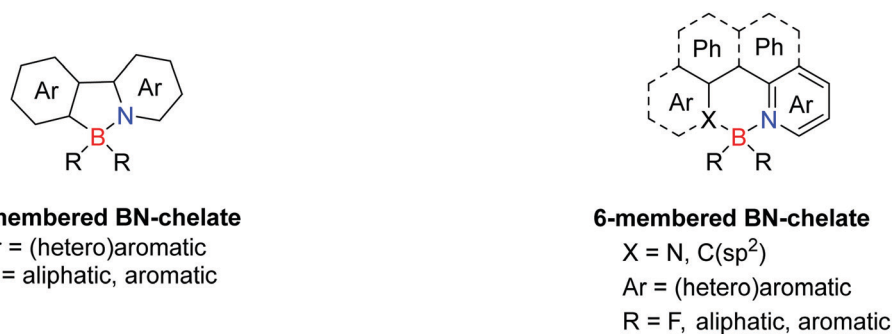
Fig. 40 Two types of four-coordinated boron-doped PAHs.
