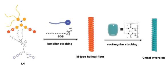
Scheme 1 A schematic diagram of the possible supramolecular assembly route for L4/SDS/CB[8] systems. SDS molecules coassembled with L4 molecules to form a binary L4/SDS supramolecule and generated the M-type helical fibers via lamellar stacking, Adding CB[8] to the L4/SDS system resulted in a new ternary L4/SDS/CB[8] supramolecular structure possessing a rectangular stacking arrangement, which also caused a chirality inversion
