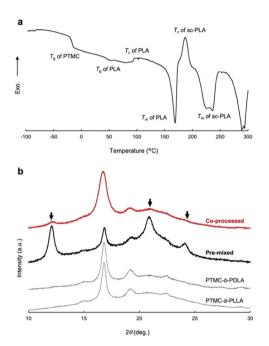
Fig. 4 (a) DSC thermograph of a co-processed extrudate of PTMC-b-PLLA(46) ( $M_{\rm w}$  121 kDa) and PTMC-b-PDLA(46) ( $M_{\rm w}$  105 kDa). (b) XRD spectra of various degradable block copolymers. Top to bottom: co-processed PTMC-b-PLLA(46) and PTMC-b-PDLA(46), pre-mixed PTMC-b-PLLA(46) and PTMC-b-PDLA(46).
