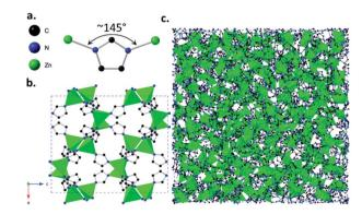
Fig. 1 (a) Zn-Im-Zn angle of ZIF-4(Zn) [Zn(Im)<sub>2</sub>] structural unit, (b) crystalline structure of ZIF-4(Zn) with unit cell parameters a=15.3486(14), b=15.1069(17), c=18.3430(19), Pbca, cag topology, (c) atomic configuration of melt-quenched  $a_{\rm g}$ ZIF-4(Zn), where  $a_{\rm g}$  denotes the glass phase. Configuration parameters: a=b=c=47.5225 Å, P1. CIFs obtained from ref. 9 and 11 respectively.
