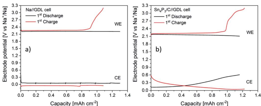
Fig. 7 Galvanostatic curves for each electrode of the Na//GDL (a) and Sn<sub>4</sub>P<sub>3</sub>/C//GDL cells (b) corresponding to the first discharge (black) and charge (red) curves during the EIS measurements. WE refers to the working electrode, *i.e.*, the cathode and CE to the counter, *i.e.*, the anode.
