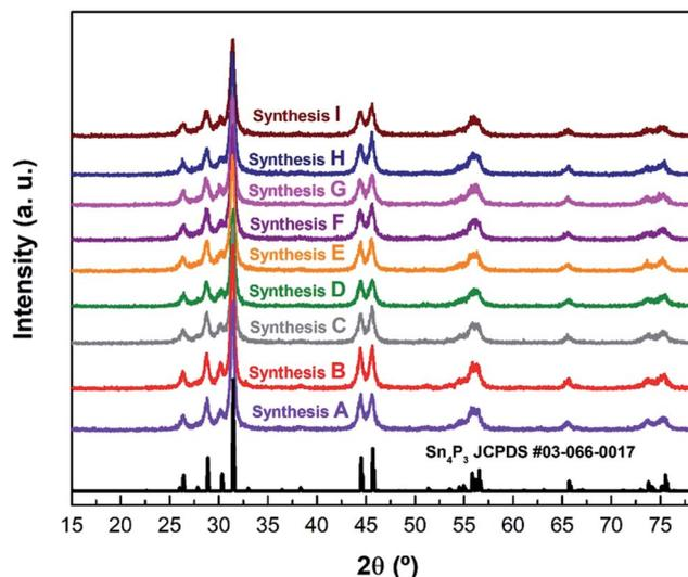
Fig. 1 The XRD patterns of the different syntheses of  $\text{Sn}_4\text{P}_3/\text{C}$  samples listed in Table 1 along with the reference pattern of  $\text{Sn}_4\text{P}_3$  (JCPDS #03-066-0017).
