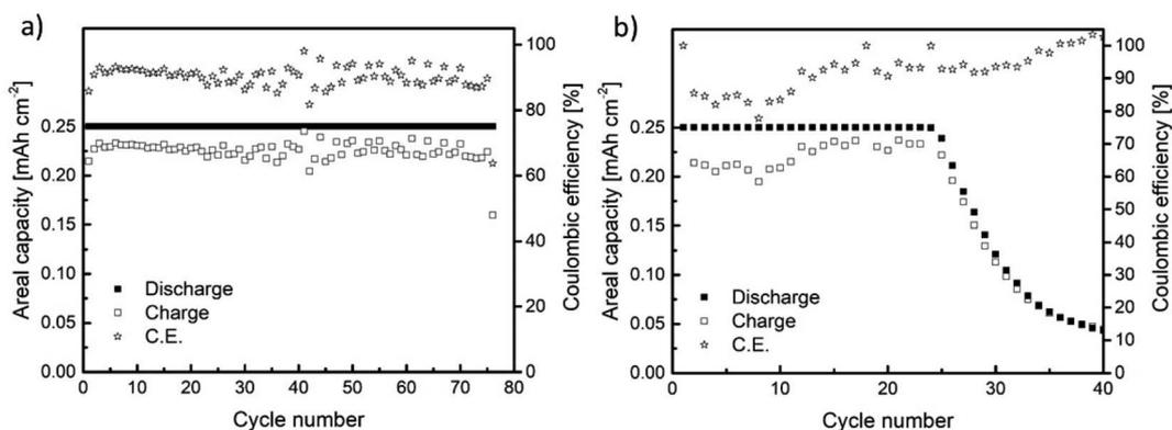
Fig. 6 Galvanostatic charge/discharge results for the cells assembled using (a) metallic Na (Na//GDL) and (b)  $\text{Sn}_4\text{P}_3$  ( $\text{Sn}_4\text{P}_3/\text{C}/\text{GDL}$ ) negative electrodes.
