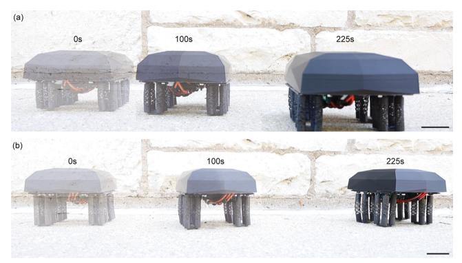
Fig. 6 Untethered soft robotic guadrupeds. Untethered HSA-based soft robots constructed with the (a) 0.5× legs and (b) stilled 0.5× legs are shown walking on a concrete sidewalk. Overlays of the quadrupeds are shown at 0 s, 100 s, and 225 s of the walking sequence. Stills are taken from Movie S4 in the ESI,† Scale bars are 50 mm.
