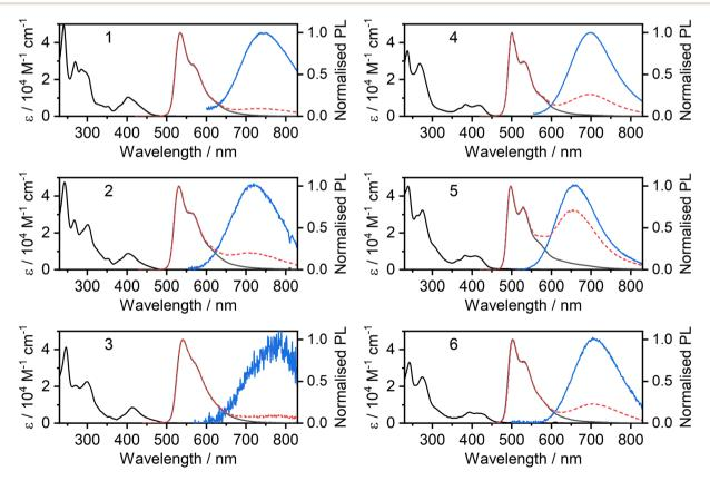
Fig. 2 Photoluminescence of complexes 2, 3, 5, and 6 in  $CH_2Cl_2$  solutions: absorption (black lines) and photoluminescence (grey) spectra in dilute ( $\approx 10^{-5}$  M) solution; photoluminescence spectra at higher concentration ( $\approx 10^{-4}$  M, dashed red); deconvoluted excimer spectrum (blue).
