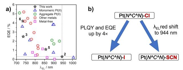
Fig. 10 (a) Maximum external quantum efficiency (EQE) and electroluminescence spectrum maxima ( $\lambda_{EL}$ ) of sample NIR OLEDs from the literature that use platinum(II) complexes or others as emitters indicated in the figure legend. See Table S7.1 in the ESI† for corresponding references. (b) Effects of the -X monodentate ligand on photoluminescence in film and electroluminescence.
