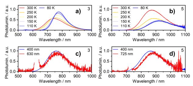
Fig. 5 Photoluminescence of complexes 3 and 5 in neat thermally deposited films: (a and b) PL spectra recorded at temperatures from 300 K to 80 K with 365 nm excitation wavelength; (c and d) PL spectra recorded at room temperature with long and short wavelength excitation as indicated in figure legend.
