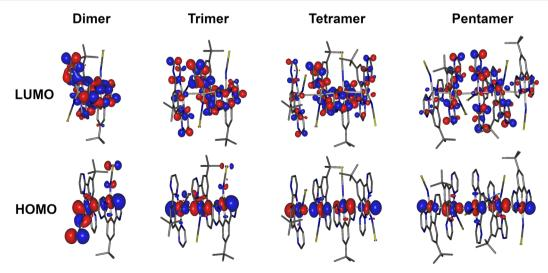
HOMO and LUMO iso surfaces in dimers, trimers, tetramers, and pentamers of complex 5(N-bound form) calculated at the T<sub>1</sub> geometry.
