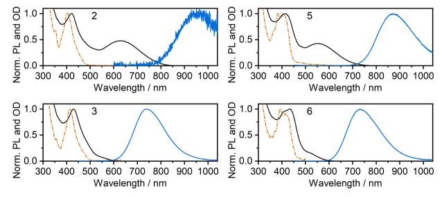
Fig. 4 Photoluminescence (blue lines) and absorption spectra (black lines) of complexes 2, 3, 5, and 6 in thermally evaporated neat films. Absorption spectra in dilute  $CH_2Cl_2$  solution (orange dashed and dotted line) from Fig. 2 are reproduced for comparison.
