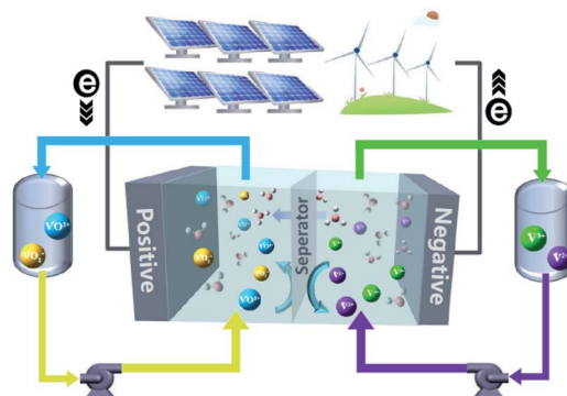
Fig. 1 A schematic diagram of a VFB.
