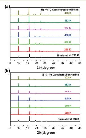
Fig. 4 Phase transitions of R-CSAI and S-CSAI. (a) Variable-temperature PXRD patterns of R-CSAI. (b) Variable-temperature PXRD patterns of S-CSAL
