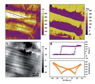
Fig. 6 Ferroelectric domains. The diagrams of (a) lateral amplitude, (b) phase, (c) topology and (d) switching spectroscopy of the S-CSAI thinfilm taken by PFM.
