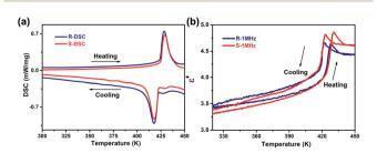
Fig. 3 Phase transitions of R-CSAI and S-CSAI. (a) DSC curves in a heating-cooling run. (b) Temperature-dependent  $\varepsilon'$  at 1 MHz upon heating and cooling.
