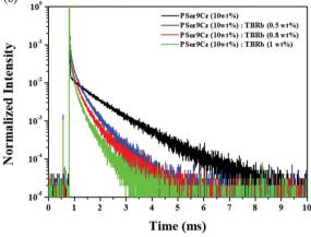
Fig. 2 (a) UV-vis absorption spectra of TBRb and fluorescence spectra of 10 w% PSez9Cz doped in the mixed host with and without TBRb dopant. The doping concentration of the fluorescent dopant was 0.5, 0.8, and 1 wt%. The mixed host was composed of mCP and TSPO1 in 50:50. (b) TRPL curves of 10 wt% PSez9Cz doped in the mixed host with and without TBRb dopant. The detection wavelength was 560 nm for the fluorescence emission peak
