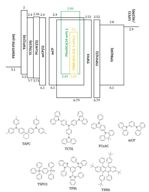
Fig. 4 Device structure of RTPH sensitized yellow fluorescent OLEDs and molecular structures of organic layer materials. The doping concentrations of TBRb were 0.5, 0.8 and 1 wt%, and that of PSez9Cz was 10 wt%.
