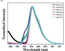
Fig. 5 (a) EQE-Luminance curve and (b) EL spectra curves at 500 cd m<sup>-2</sup> of RTPH sensitized yellow hyperfluorescent OLEDs.
