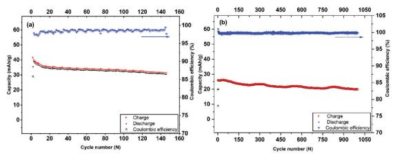
Fig. 6 Long-term cycling performance and coulombic efficiency of  $Mo_6S_8$  nanocubes at 0.2 C-rate (a), and 4 C-rate (b).
