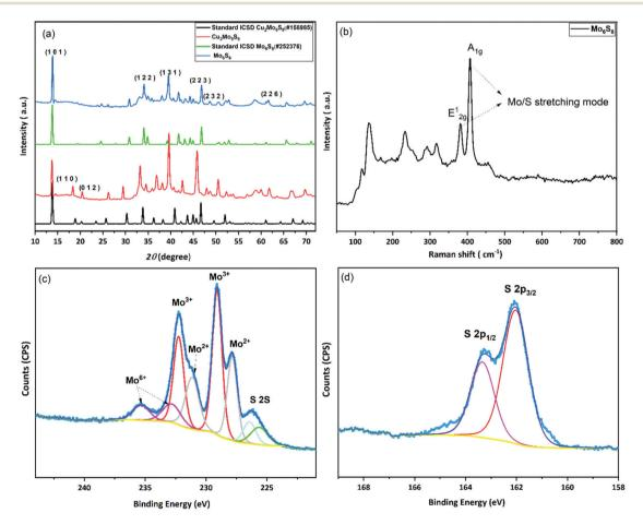
Fig. 1 Characterization of the prepared materials: (a) P-XRD pattern of the as-synthesized Cu<sub>2</sub>Mo<sub>6</sub>S<sub>8</sub> and Mo<sub>6</sub>S<sub>8</sub> along with their corresponding standard patterns, (b) Raman spectrum of Mo<sub>6</sub>S<sub>8</sub>, (c) high resolution XPS spectra of the Mo 3d/S 2s region and (d) S 2p region.
