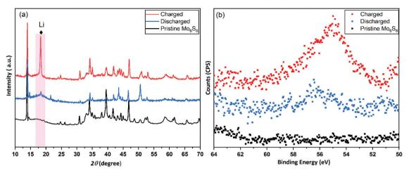
Fig. 7 Post-mortem characterization on cycled  $Mo_6S_8$  electrodes. (a) Post-mortem P-XRD characterization was conducted on the pristine, fully charged to 2.2 V, and fully discharged to 0.5 V  $Mo_6S_8$  electrode. (b) High resolution XPS spectra of the Li 1s for the pristine, charged, and discharged  $Mo_6S_8$  electrode.
