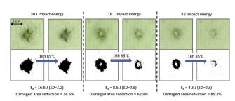
Fig. 14 Image analysis of the healing of low-velocity impact at 3 different levels of impact energy. Healing is performed at 85 °C and under 0.02 MPa for 16 h. Top images show the real damaged composite whereas the bottom pictures show the same pictures treated with a binary filter to facilitate characterization. Reproduced with permission from ref. 79. Copyright 2017 Elsevier Ltd.
