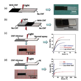
Fig. 7 Transmission welding (a) joining a non-CNT vitrimer with a CNTvitrimer. (b) Joining two pieces of a non-CNT vitrimer using a CNT-vitrimer as an "adhesive". (c) Joining normal epoxy with a CNT-vitrimer. (d) Joining thermoplastic PE with a CNT-vitrimer. Reproduced with permission from ref. 64. Copyright The Royal Society of Chemistry 2014.
