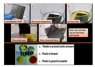
Fig. 20 Recycling of Mallinda's CFRP vitrimer. 99
