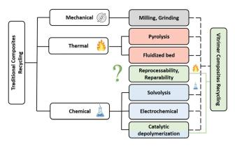
Fig. 1 Classification of the major recycling methods of traditional composites with possible alternatives offered by vitrimer composites.
