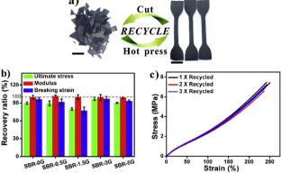
Fig. 11 (a) Optical images showing the recycling of SBR-3G, and the scale bar represents 1 cm; (b) recovery ratio of the mechanical performance of SBR-xG between the first and second generations of recycling; and (c) stress-strain curves of SBR-3G after multiple cycles of recycling. Reproduced with permission from ref. 69. Copyright 2018 Elsevier Ltd.
