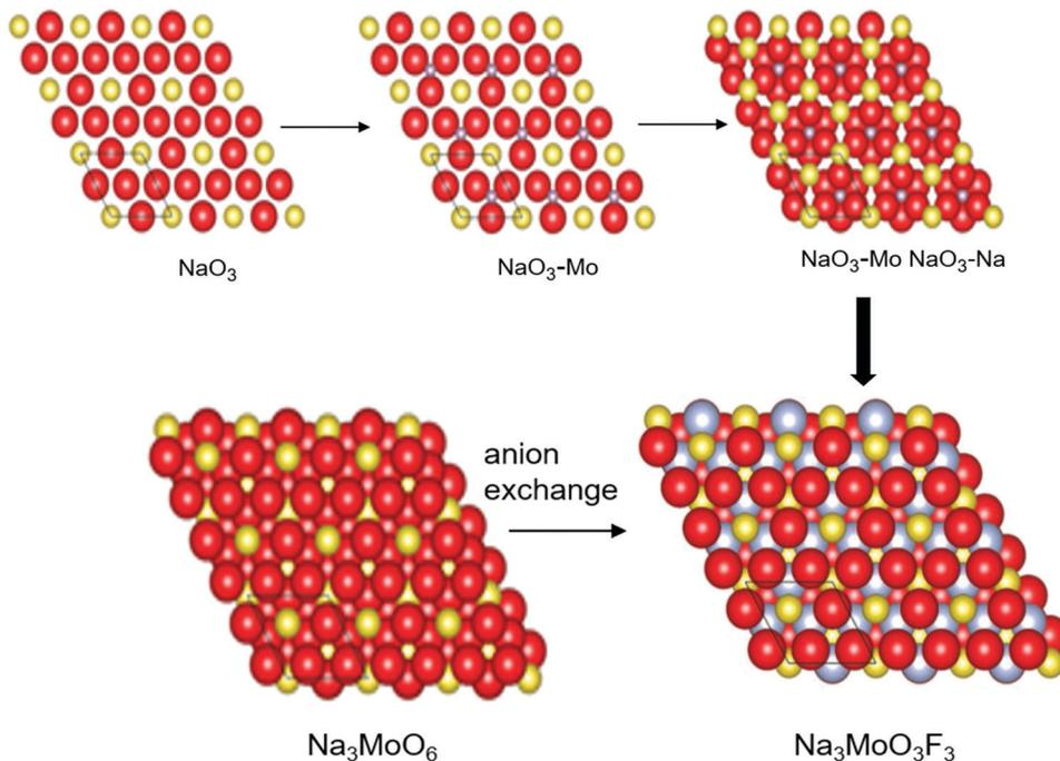
Fig. 5 Construction of the heteroanionic materials  $\text{Na}_3\text{MoO}_3\text{F}_3$ . Computational analysis helps in predicting building units  $\text{NaO}_3\text{F}_3$  and  $\text{MoO}_3\text{F}_3$  and their arrangements in the cluster. This type of heteroanionic arrangement alters the electronic, magnetic, and optical properties of molecules (reproduced with permission from ref. 11).
