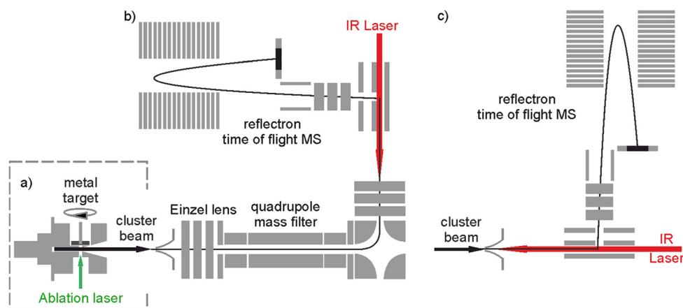
Fig. 1 Schematic of the instruments used for infrared action spectroscopy of  $[\text{HoO}_m(\text{CO}_2)_n]^+$  complexes. The cutaway source, (a), is common to both experiments. In variant (b) a quadrupole mass filter–bender assembly (Extrel) provides parent ion mass selection. In (c) IR-induced depletion of a wide range of Ar-tagged complexes is recorded simultaneously. In both cases infrared excitation occurs before detection.
