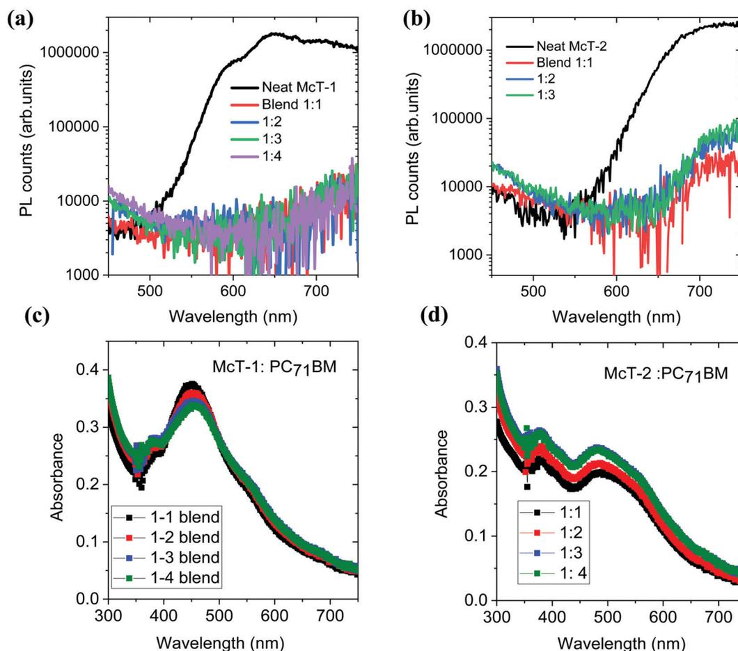
Fig. 8 Steady state photoluminescence spectra of (a) neat **McT-1** and blend with **PC<sub>71</sub>BM** for different ratios (b) neat **McT-2** and blend with **PC<sub>71</sub>BM** for different ratios. The excitation wavelength is 450 nm. Absorbance spectra of the (c) **McT-1** and **PC<sub>71</sub>BM** blends (d) **McT-2** and **PC<sub>71</sub>BM** blends as a function of different blend ratios.
