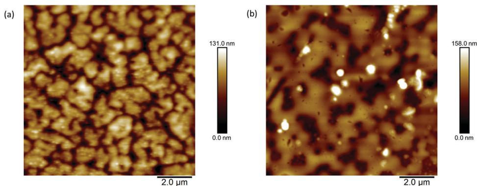
Fig. 7 Tapping mode atomic force microscopy images of **McT-1** films deposited from (a) chloroform (RMS roughness = 17.8 nm) and (b) toluene (RMS roughness = 22.8 nm) solutions on prefabricated OFET substrates. Scan area =  $10 \times 10 \mu\text{m}^2$ .
