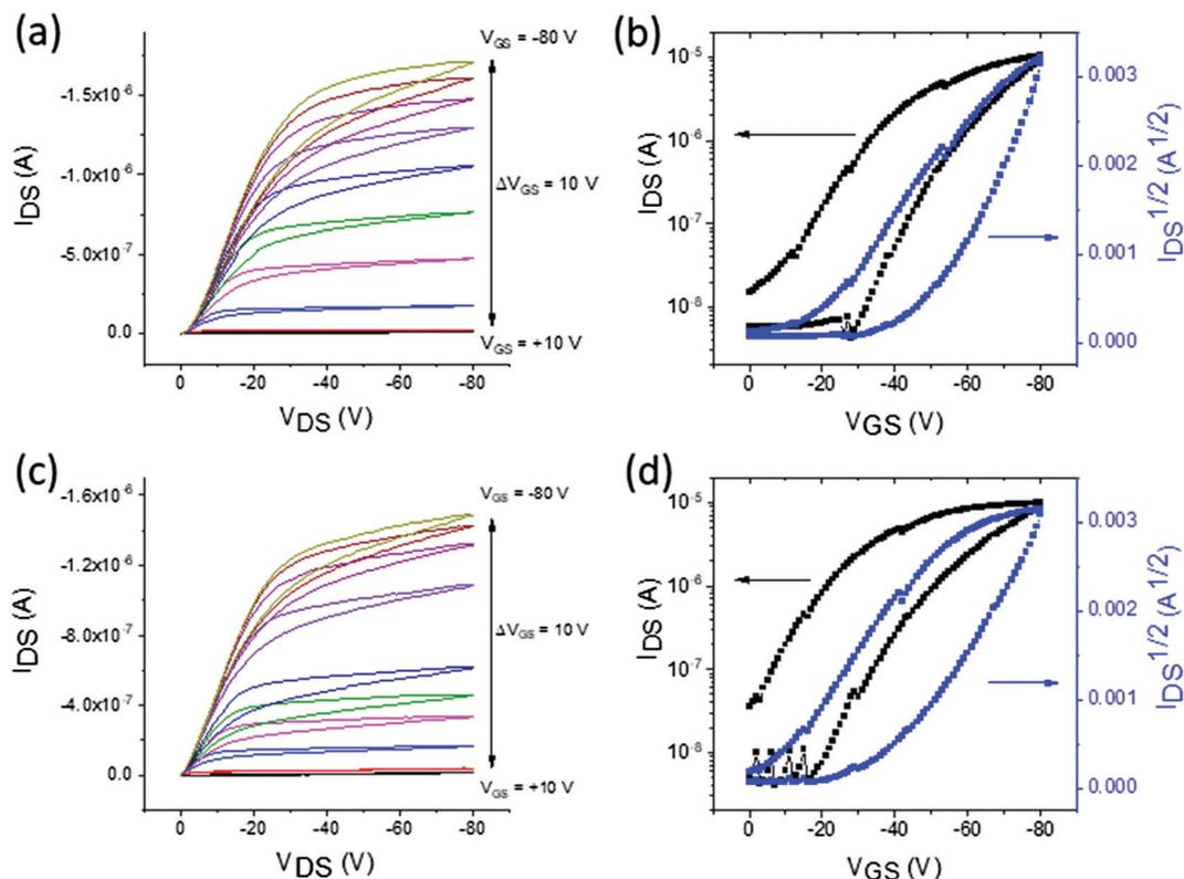
Fig. 6 Characterisation of OFETs fabricated using **McT-1**, channel length = 10  $\mu\text{m}$ , channel width = 1cm. Output characteristics of OFETs fabricated using **McT-1** in (a) chloroform and (c) toluene solutions. Transfer graphs for **McT-1** films deposited using (b) chloroform and (d) toluene solutions where  $V_{\text{DS}} = -70$  V.
