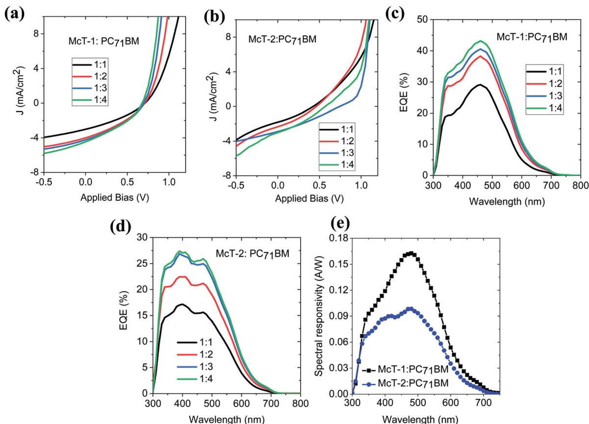
Fig. 9  $J$ - $V$  characteristics of the (a) **McT-1:PC<sub>71</sub>BM** and (b) **McT-2:PC<sub>71</sub>BM** blends as a function of different blend ratios. External quantum efficiency (EQE) spectra of the (c) **McT-1:PC<sub>71</sub>BM** and (d) **McT-2:PC<sub>71</sub>BM** blends as a function of different blend ratios. (e) Spectral responsivity curves of the corresponding photovoltaic devices estimated from their EQE spectra.
