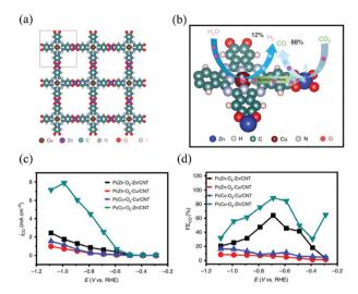
Fig. 5 Cu<sup>II</sup>-Zn<sup>II</sup> bimetallic coordination polymers as a CO<sub>2</sub> reduction electrocatalyst: (a) packing structure, (b) a proposed synergistic catalytic scheme based on DFT calculations, (c) partial current and (d) Faraday efficiency of CO production at different potentials. Adapted from ref. 89.
