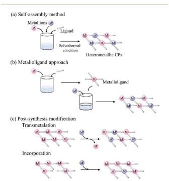
Fig. 1 General synthesis methods for heterometallic coordination polymers: (a) self-assembly method, (b) metalloligand approach, and (c)
