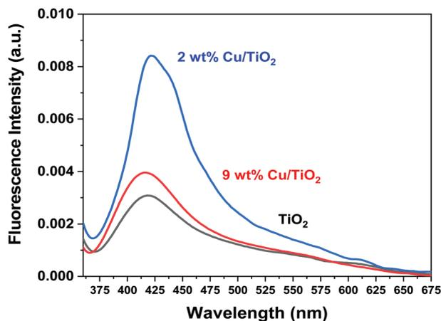
**Fig. 11** Photoluminescence spectra of the obtained bare TiO<sub>2</sub> and titania modified with Cu (2 and 9 wt%), when excited at 340 nm.
