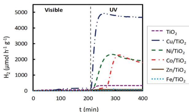
**Fig. 2** Hydrogen production for impregnated M/TiO<sub>2</sub> photocatalysts (M = Fe, Co, Ni, Cu, Zn), 2 wt% M, under both visible and UV light irradiation.
