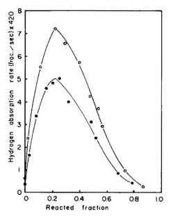
Fig. 5 Hydrogen absorption rate as a function of reacted fraction at 20 °C. The curve with black dots was obtain under 20 bar of hydrogen, whereas the one with white dots under 24 bar. Reproduced with permission from ref. 94
