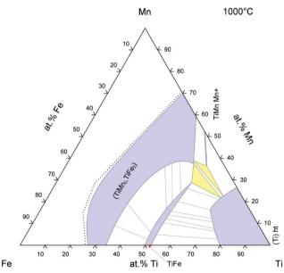
Fig. 6 Isotherm section at 1000  $^{\circ}$ C of the Ti–Fe–Mn phase diagram. Reproduced with permission from ref. 22.
