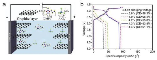
Fig. 32 (a) Operation principle of the DIB containing  $(DMPI^+)(AlCl_4^-)$  as an IL electrolyte. (b) Charge/discharge curves of the DIB cell at cut-off charging voltages of 3.8–4.4 V. Reproduced from ref. 439 with permission from Elsevier.
