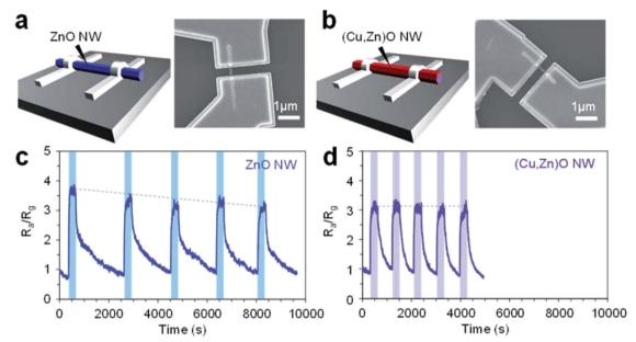
Fig. 9 (a and b) Schematic and SEM images of single nanowire sensor devices using the (a) ZnO nanowire and (b) (Cu,Zn)O nanowire.<sup>99</sup> (c and d) Five successive sensor responses to nonanal using the ZnO nanowire device and (Cu,Zn)O nanowire device, respectively.<sup>99</sup>
