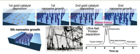
Fig. 7 The 3D nanowire array for ultra-fast separation of biomolecules. 79 The 3D nanowire array was fabricated by repeating catalyst deposition on the targeted special location and nanowire growth from the deposited catalyst.
