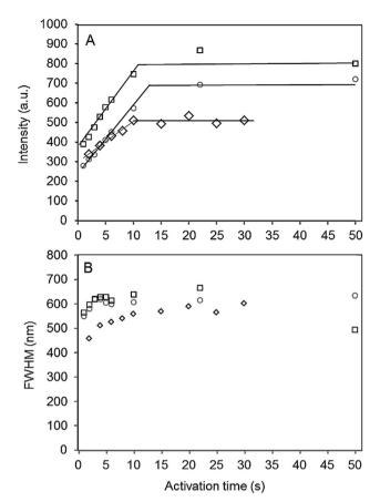
Fig. 2 Intensity (A) and FWHM (B) of photo-activated carbon nanodots, given as a function of the activation time for 3 individual AlPO-5 crystals using 9.5 MW cm<sup>-2</sup> as the activation power. The solid lines in Fig. 2A are only used to indicate the trends.
