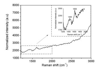
Fig. 4 Raman spectrum from 1200 to 3000 cm<sup>-1</sup> of an activated carbon nanodot in AIPO-5 after background subtraction. The inset shows an enlargement of the observed D and G-bands.
