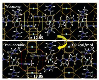
Packing interactions between imidazolium rings along the [001] channels in the tetragonal (top) or pseudocubic (bottom) cell, showing the steric repulsion in the latter case
