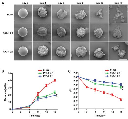
Fig. 3 Degradation properties of PLGA, P/C-h 4:1, and P/C-h 2:1 microparticles. (A) SEM images of the microparticles. Scale bars = 20 μm. (B) Weight loss of microparticles immersed in PBS for 0, 3, 6, 9, 12 and 15 days. (C) The pH value changes of the solutions immerging the microparticles for 0, 3, 6, 9, 12 and 15 days. The data were reported as the mean  $\pm$  SD, n=5. \*\*\* significant difference, p<0.001. \*\* significant difference, p<0.01.
