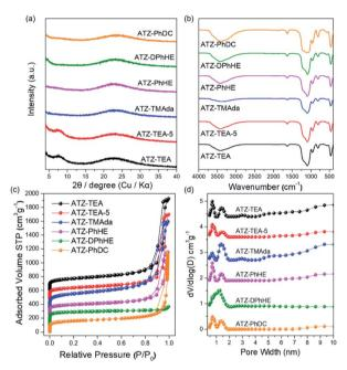
Fig. 1 (a) XRD patterns, (b) FT-IR spectra, (c)  $\rm N_2$  adsorption and desorption isotherms, and (d) pore size distributions of the ATZ samples.
