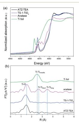
Fig. 4 (a) Ti K-edge XANES spectra and (b) Fourier transform  $k^2$ -weighted Ti EXAFS spectra in the R spacing of the ATZ-TEA sample, TS-1-TiO<sub>4</sub> zeolite sample, anatase TiO<sub>2</sub>, and Ti foil reference.
