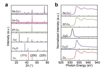
Fig. 2 Structural characterization of EP-Cu, Ox-Cu and Re-Cu-I. (a) GIXRD patterns of Re-Cu-I (purple), Ox-Cu (pink), EP-Cu (yellow) and reference samples CuI (black, PDF#06-0246), Cu<sub>2</sub>O (blue, PDF#05-0667), and Cu (red, PDF#04-0836). (b) Cu L-edge XAS spectra of Re-Cu-I (purple), EP-Cu (yellow) and reference samples CuO (black), Cu<sub>2</sub>O (blue) and Cu (red).
