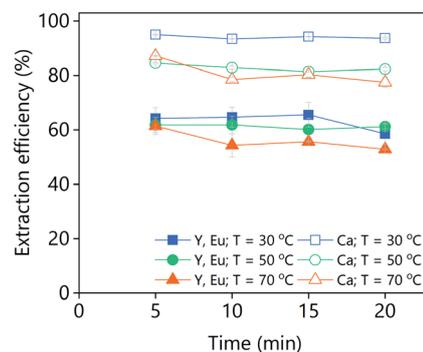
Fig. 13 Stripping efficiency *via* oxalic acid addition (stoichiometric amount) as a function of time and temperature of a levulinic acid PLS obtained from the leaching of real lamp phosphor residue. The leaching conditions are:  $\text{H}_2\text{O}$  vol% = 30;  $T = 80$  °C;  $t = 48$  h;  $L/S = 10$ ; and 500 rpm.
