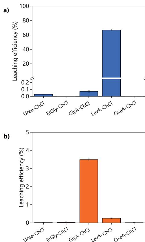
Fig. 2 Effect of the hydrogen-bond donor type on the leaching efficiency of (a) YOX lamp phosphor and (b) HALO lamp phosphor. The leaching conditions are:  $\text{H}_2\text{O}$  vol% = 10;  $T = 80^\circ\text{C}$ ;  $t = 48$  h;  $L/S = 10$  and 500 rpm.
