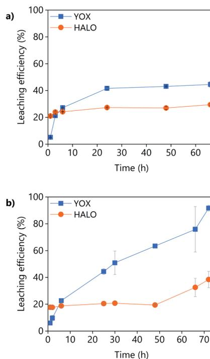
**Fig. 8** Effect of the leaching time on the leaching efficiency of a real lamp phosphor waste using (a) LevA–ChCl and (b) levulinic acid. The leaching conditions are: H<sub>2</sub>O vol% = 30; T = 80 °C; L/S = 10; and 500 rpm.
