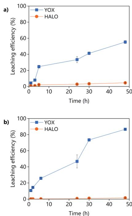
Fig. 7 Effect of the mixing time on the leaching efficiency of a synthetic lamp phosphor mixture using (a) LevA–ChCl and (b) levulinic acid. The leaching conditions are: H<sub>2</sub>O vol% = 30; *T* = 80 °C; L/S = 10; 500 rpm.
