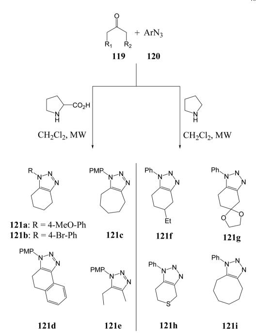
Scheme 10 Synthesis of 1,2,3-triazole derivatives via unactivated ketones. 103
