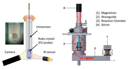
Fig. 2 (Left); scheme of a monomode reactor. (Right); scheme of a multi-mode reactor. (16)
