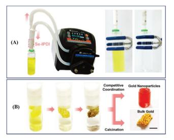
Fig. 11 (A) The equipment for simulating the dynamic extraction process in industrial treatment and the color change of the Au<sup>3+</sup> solution before and after treatment with the system; (B) procedure of gold extraction with Se-foam and posttreatments by competitive coordination or calcination. Reproduced with permission from ref. 216. Copyright 2020 WILEY-VCH Verlag GmbH & Co. KGaA, Weinheim.
