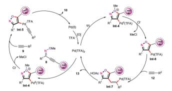
Scheme 6 Plausible mechanism for palladium-catalyzed cyclization/ alkynylation and alkenylation.
