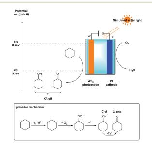
Scheme 5 PEC cells for C-H bond activation of cyclohexane
