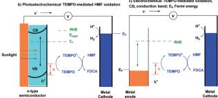
Scheme 2 Schematic comparison of photoelectrochemical and electrochemical cells.
