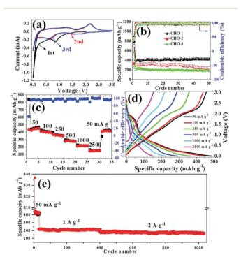
Fig. 9 (a) CV curves of CHO-1 and (b) cycling performance of CHO electrodes at a current density of 50 mA  $\rm g^{-1}$ . (c) Rate capabilities at different current densities, (d) typical discharge—charge curves at different current densities and (e) long cycling performance of CHO-1. The CHO samples obtained from pyrolysis of MOFs at 300, 350 and 400 °C are denoted as CHO-1, CHO-2 and CHO-3, respectively. Reproduced from ref. 71 with permission from the Royal Society of Chemistry.
