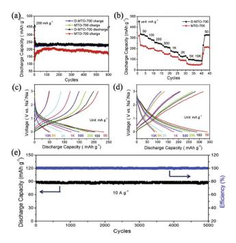
Fig. 7 (a) Cycling performance of MTO-700 (regular TiO<sub>2</sub>/carbon) and D-MTO-700 (defect-rich TiO<sub>2</sub>/carbon). (b) Rate performance of MTO-700 and D-MTO-700 at various current densities. Charge-discharge curves of MTO-700 (c) and D-MTO-700 (d) at various current densities. (e) Cycling performance of D-MTO-700. Reprinted from ref. 55, Copyright (2017), with permission from Elsevier.
