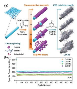
Fig. 4 (a) Preparation of hierarchical CoCHs derived from M(MOFs) @PAN fibers. (b) Cycle performance of CoCHs in SIBs at 100 mA  $q^{-1}$ . Reproduced from ref. 39 with permission from John Wiley and Sons.
