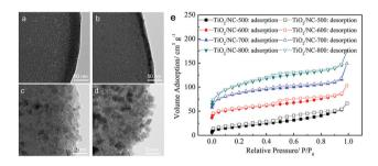
Fig. 6 TEM images of (a) TiO<sub>2</sub>/NC-500, (b) TiO<sub>2</sub>/NC-600, (c) TiO<sub>2</sub>/ NC-700, (d)  $TiO_2/NC-800$  and (e)  $N_2$  sorption isotherms of the four nanocomposites prepared at different temperatures. Reproduced from ref. 59 with permission from John Wiley and Sons.
