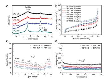
Fig. 2 (a) X-ray diffraction (XRD), (b) N<sub>2</sub> sorption isotherms, (c) rate capability and (d) cycling performance of the ZIF-67-derived carbons pyrolyzed at temperatures from 600 to 900 °C. Reproduced from ref. 45 with permission from John Wiley and Sons.
