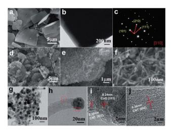
Fig. 8 (a) SEM image, (b) TEM image, and (c) selected area electron diffraction analysis of Co-MOFs. (d-f) SEM images of CoO-NCNTs at different magnifications. (g and h) TEM and (i and j) HRTEM images of CoO-NCNTs corresponding to the two marked regions in (h). Reproduced from ref. 67 with permission from the Royal Society of Chemistry.
