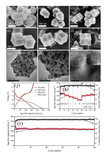
Fig. 15 FESEM images of (a and b) ZIF-67, (c and d) Co@PCP and (e and f) CoSe@PCP at different magnifications. (g, h and i) HRTEM images of CoSe@PCP at different magnifications. (j) Galvanostatic charge and discharge profiles in the 1st, 2nd, 3rd and 50th cycles at 100 mA  $g^{-1}$ . (k) Rate performance and (I) cycling performance at 100 mA q<sup>-1</sup> of CoSe@PCP. Reprinted from ref. 115, Copyright (2017), with permission from Elsevier.
