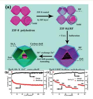
Fig. 14 (a) Schematic illustration of the synthesis process. (b) Cycling performance (at 100 mA g<sup>-1</sup>) and (c) rate capability of the ZnS-Sb<sub>2</sub>S<sub>3</sub>@C core-shell SIB anodes. Adapted with permission from ref. 28. Copyright (2018) American Chemical Society.
