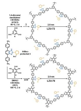
Fig. 16 Schematic presentation of the synthesis of LZU-72 and LZU-76.
