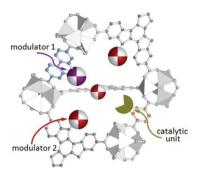
Fig. 11 Schematic depiction of a pore in MUF-77 equipped with a site for catalysis and modulator groups that are positioned to modulate the environment of the reaction.
