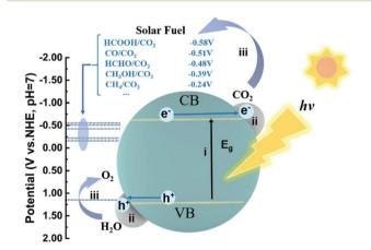
Fig. 1 Schematic illustration of the overall process for photocatalytic CO<sub>2</sub> reduction with H<sub>2</sub>O over a semiconductor photocatalyst. The dotted lines indicate the thermodynamic potentials for water oxidation into O2 and CO2 reduction into CH4, CH3OH, HCHO, CO and HCOOH, respectively. The numbers i, ii and iii represent the three critical steps in photocatalytic CO<sub>2</sub> reduction.
