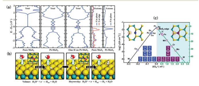
Fig. 2 (a) DOS of MoS<sub>2</sub>, Pt-MoS<sub>2</sub>, and H adsorbed Pt-MoS<sub>2</sub>. The dashed line represents the Fermi level. (b) HER process through the Volmer-Heyrovsky pathway on a Pt-MoS<sub>2</sub> catalyst. (c) Volcano plot of  $2H-MoS_2$  doped with different transition metals at the Mo substitution site.  $^{26}$
