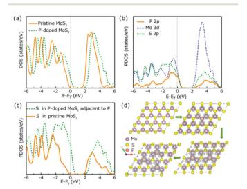
Fig. 5 (a) Total DOS of pure MoS<sub>2</sub> and P doped MoS<sub>2</sub>. (b) Partial DOS of P-MoS<sub>2</sub>. (c) Partial DOS for S atoms. The vertical grey lines represent the Fermi level. (d) Partial charge density of P-MoS<sub>2</sub> when doped with 0-3 P
