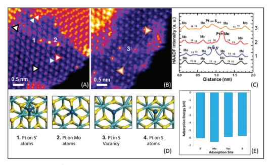
Fig. 4 (a) and (b) HAADF-STEM of Pt-1T- $^{S}$ MoS<sub>2</sub>. (c) ADF intensity line profiles taken along the corresponding coloured line of black, blue, red, and orange in the  $\langle 110 \rangle$  direction. (d) The proposed model of the Pt atom doping at 4 different adsorption sites. Numbers 1, 2 and 3 correspond to the experimentally observed Pd position shown in (a) and (b). (e) Adsorption energy for Pt atoms on each proposed adsorption site.<sup>29</sup>
