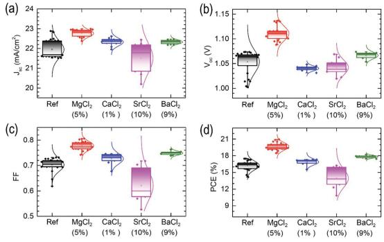
Fig. 2 Statistical photovoltaic parameters of (a)  $V_{\rm sc}$ , (b)  $V_{\rm oc}$ , (c) FF and (d) PCE measured at reverse scan for the BCl<sub>2</sub> additives (B = Mg, Ca, Sr and Ba). Values in parentheses are the optimal mol% of the additive with respect to FAPbl<sub>3</sub>.
