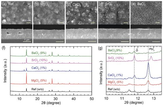
Fig. 3 (a-e) Top-view and cross-sectional scanning electron microscope (SEM) images and (f, g) X-ray diffraction patterns of FAPbI $_3$  films with and without (Ref) additives of MgCl $_2$ , CaCl $_2$ , SrCl $_2$  and BaCl $_2$ .
