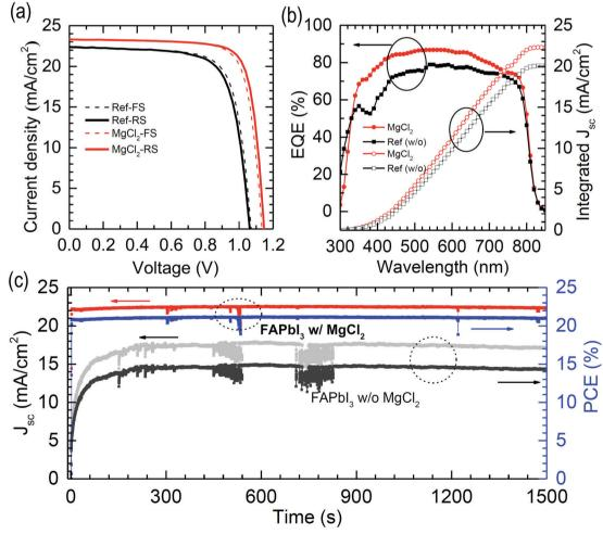
Fig. 8 (a) J-V curves and (b) external quantum efficiency (EQE) of PSCs employing FAPbl<sub>3</sub> with and without MgCl<sub>2</sub> additive. (c) Steady-state  $J_{sc}$  and PCE for the PSCs employing FAPbl<sub>3</sub> with and without the MgCl<sub>2</sub> additive, measured at the maximum power point (MPP) for 1500 s under continuous 1 sun illumination.
