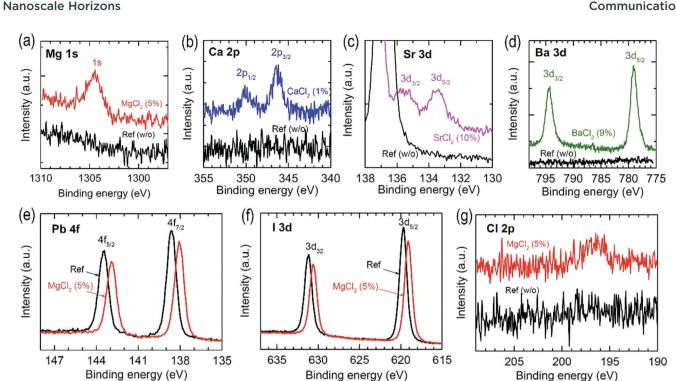
Fig. 5 Mg 1s, Ca 2p, Sr 3d and Ba 3d X-ray photoelectron spectroscopy (XPS) spectra of the annealed FAPbI<sub>3</sub> films with and without additives of (a) MgCl<sub>2</sub>, (b) CaCl<sub>2</sub>, (c) SrCl<sub>2</sub> and (d) BaCl<sub>2</sub>. (e) Pb 4f, (f) I 3d and (g) Cl 2p XPS spectra of the FAPbl<sub>3</sub> films before and after adding the MgCl<sub>2</sub> additive.
