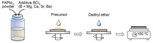
Fig. 1 A schematic illustration of the perovskite deposition procedure. The precursor solution was prepared by mixing the pre-synthesized FAPbl<sub>3</sub> powder with BCl<sub>2</sub> additive (B = Mg, Ca, Sr and Ba), which was spin-coated. Diethyl ether was dipped for 20 s after rotating the substrate. The film was annealed at 150 °C in an air atmosphere
