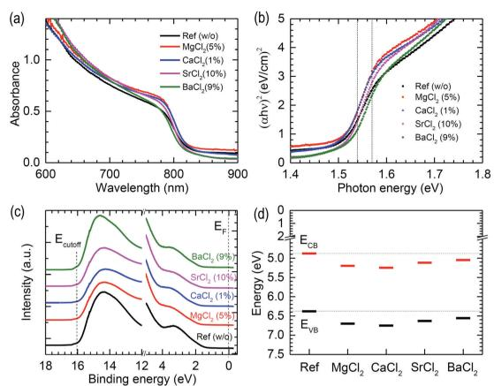
Fig. 6 (a) UV-vis spectra, (b) Tauc plot, (c) ultraviolet photoelectron spectroscopy (UPS) and (d) band (conduction band (CB) and valence band (VB)) positions for the FAPbl<sub>3</sub> films with and without additives. UPS spectra were measured with He I photon energy (21.2 eV).
