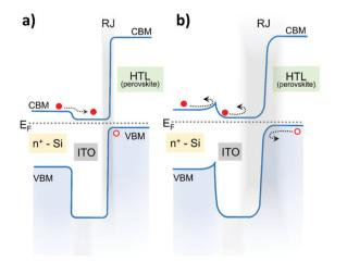
Fig. 3 Band diagram of the RJs of the silicon/perovskite tandems with (a) ideal and (b) with Fermi level pinned contacts.
