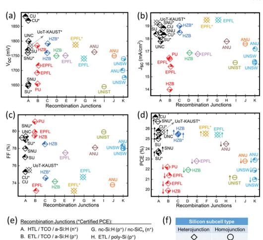
Fig. 5 (a)  $V_{\rm OC}$ , (b)  $J_{\rm SC}$ , (c) FF and (d) PCE values of the reported silicon/perovskite monolithic tandem solar cells with different RJs. Descriptions for the RJs (e) and tandem device indicators (f). The asterisks represent independently certified values.
